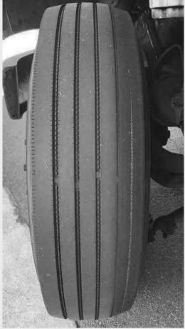
position to run, then cap the tire saving the casing. Running it into the cords ruins the tire and eliminates any casing use. These casings can be worth as much as \$200.00 each.
