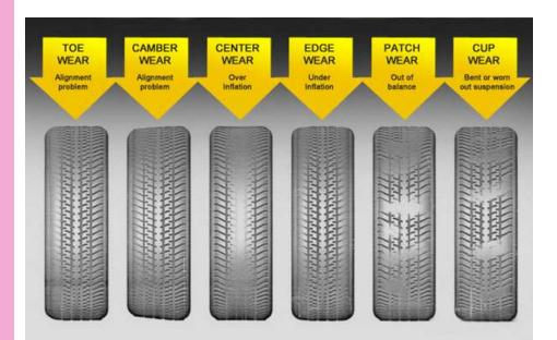
It is important to catch this wear early to possible save the tire by getting it balanced or at least being able to move it to a trailer position to run, then cap the tire saving the casing. Running it into the Cords ruins the tire and eliminates any casing use. These casings can be worth as much as \$200.00
